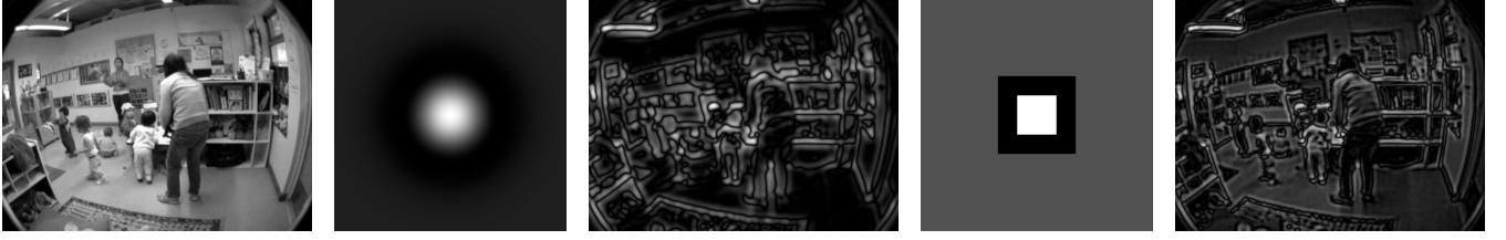
Fig. 2. Difference of Gaussians filter, and the Difference of Boxes approximation. The filters are typical of those used in this paper, with the r_{center} = 1/2 r_{surround} . The filters are respectively applied to the original image (left). Absolute filter responses are shown.
