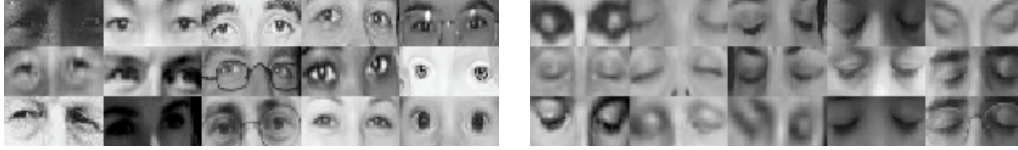
Fig. 13. Example open eyes (left) and closed eyes (right) used to train the blink detector. About 120 images of each type were taken from the web to include a wide variety of lighting conditions, facial types, glasses, and image quality. The eye detection system was used to automatically crop, scale and rotate the image patches to an upright frontal view.
