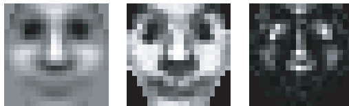
Figure 1: Left: The weights from the ridge regression network in experiment (1). Brighter pixels are more positive and darker pixels are more negative. Center: The “favorite” pixel intensities from the SNoW network in experiment (4). Notice the similarity to the ridge regression weights. Right: The sum of the weights for each pixel in SNoW. The brighter a pixel is, the more important it is for that pixel to be close to the “favorite” intensity. The high value pixels SNoW focuses on correspond to facial features such as eyes, bridge of the nose, nostrils, cheeks and forehead.
