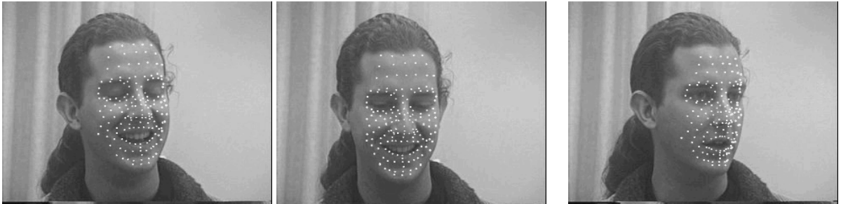
Figure 7: A demonstration of Brand's real time 3D face tracking method at work on Subject 19.
