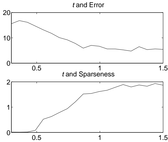
Fig. 4. The effect of control parameter t over mean square error and sparseness.
