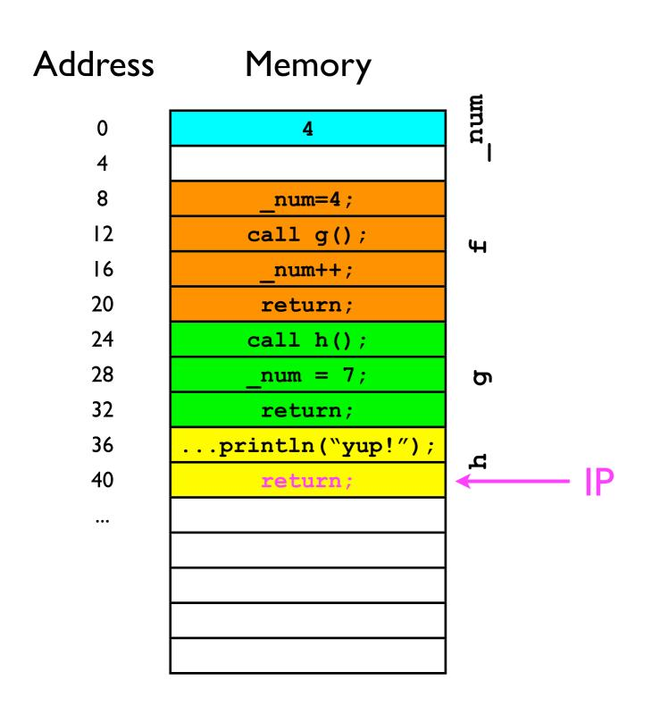
• The return call at address 40 should cause the CPU to jump to address 28 -- the next instruction in g.
