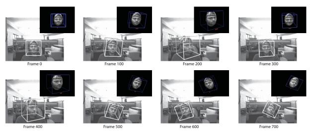
Figure 3. Head pose estimates from GAVAM depicted as a white box superimposed on the original images. In the top right corner of each image, the textured elliptical model after the completed pose estimation is shown. The thickness of cube is inversely proportional to to the variance of the pose. The small dots underneath the box represent the number of base frame used to estimate the pose.
