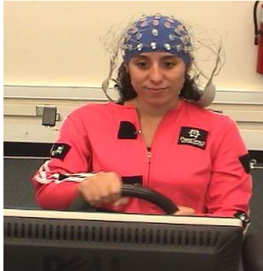
Fig. 8. Future experimental setup with the EEG and Motion Capture Systems
