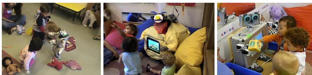
Figure 3.3: Three robot members of the RUBI project. **Left:** QRIO is a humanoid robot prototype on loan from Sony corporation. **Center:** RUBI-1, the first prototype developed at UCSD. **Right:** RUBI-3 (Asobo) the third prototype developed at UCSD. It teaches children autonomously for weeks at a time
