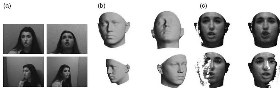
Fig. 12. Head pose estimation and warping to frontal views. (a) Four camera views of a subject at one instant. (b) Head pose estimate for each of four camera views. (c) Face images warped to frontal.
