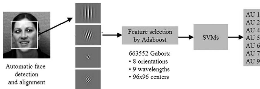
Fig. 9. Fully automated facial action coding system.
