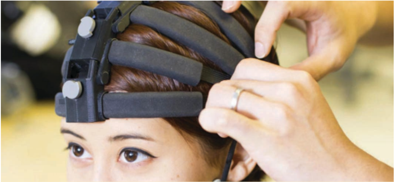
The world's first 64-channel "dry" EEG doesn't need conductive paste. (Credit: Jacobs School of Engineering)
