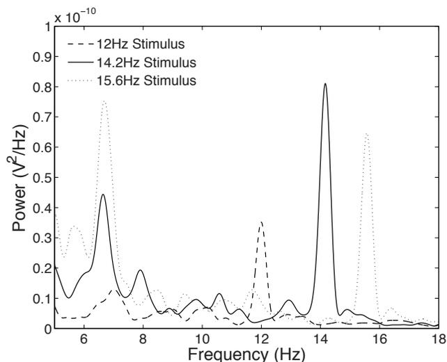
**Figure 12: Power power spectrum from the SVP experiment. The subject was asked to look at a flashing stimulus at specific frequencies. The same frequency can be observed in the occipital capacitive electrode.**
