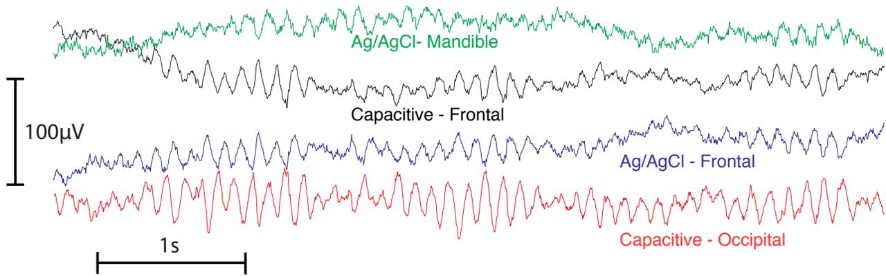
**Figure 9:** Close-up of EEG signals acquired using a mix of Ag/AgCl (3M Red Dot) and capacitive non-contact electrodes. No extra filtering beyond the analog anti-alias has been applied to the raw signal to show that the sensor is free from 60Hz interference.
