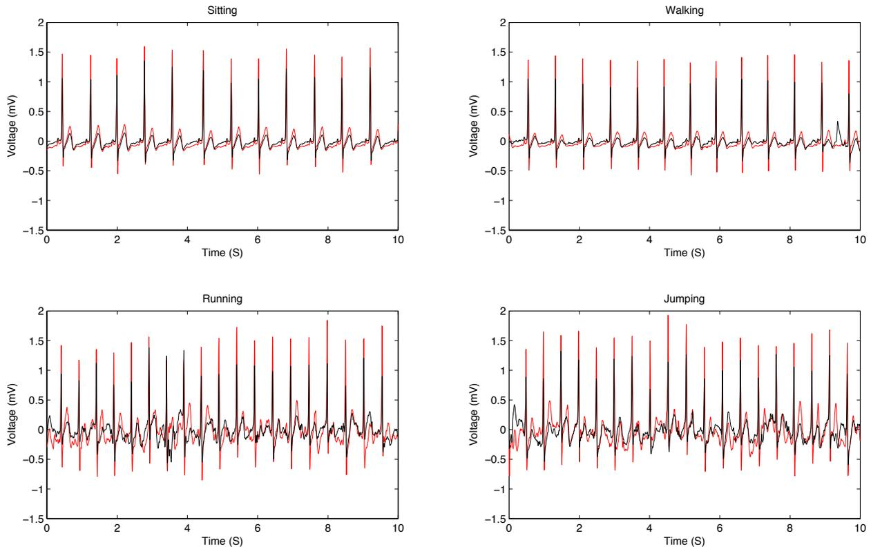
**Figure 7: A 10-second long comparison of signal from 3M Red Dot (red trace) versus non-contact electrodes (black trace) during various activities. The non-contact electrodes were fixed in a tight chest band on top of a cotton shirt.**
