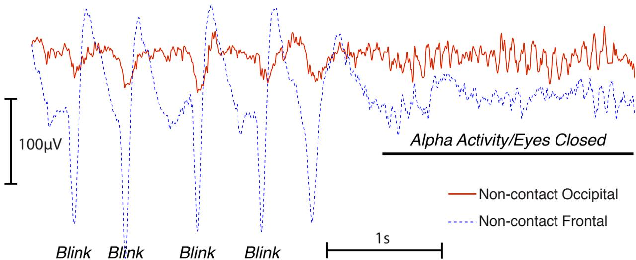
**Figure 10:** Experiment showing the signal from the frontal capacitive electrode (Fp1A1) in blue and the signal from the occipital capacitive electrode (O1A1). Eye blink artifacts are visible in the frontal electrodes during the first half of the recording. Strong alpha activity is seen in the occipital electrode after the subject's eyes close.
